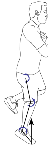
Figure 1: Sagittal plane ankle, knee, and hip joint torques (blue arrows) and vertical ground reaction force (black arrow) for one-legged hopping. The lower limbs were estimated as three-link planar systems.
