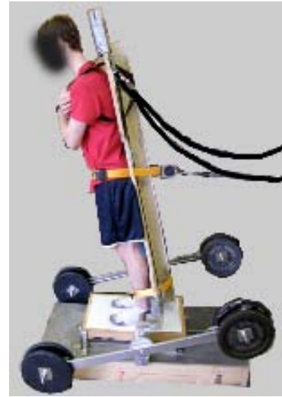
Figure 1: Experimental setup showing backboard with weights attached to arm pieces (added inertia condition shown).
