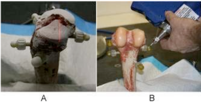
Figure 2: Laser scanning (A) and marker probing (B) with FARO arm.
