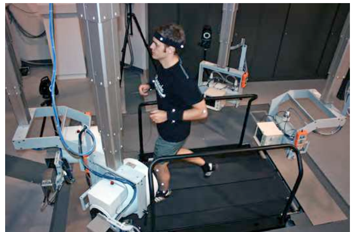
Figure 1: Dynamic Stereo X-Ray (DSX) system, configured for knee imaging during treadmill running.
