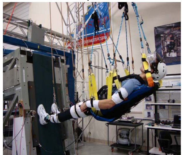
Figure 1: Subject suspended in the eZLS facility tilted to achieve 1/6 BW load at the feet.
