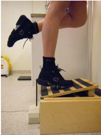
Figure 1: The heel-rise test with the linear encoder attached to the heel of the shoe.
