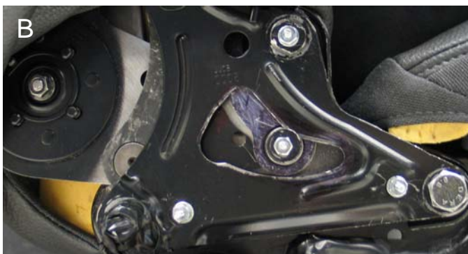
Fig. 2. A) Average motions of the right WHIPS guide pin during the 13.3 g rear crashes. B) Representative photograph of the right WHIPS recliner taken after the rear crash.
