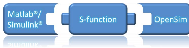
Figure 1: New S-function (system function) interface linking rapid design and control tools of MATLAB®/Simulink® with neuromusculoskeletal dynamic simulation tools of OpenSim.
