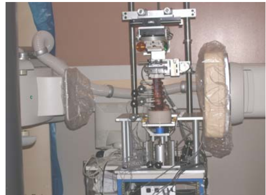
Figure 1: Cadaveric spine specimen with optoelectric sensors intact, mounted in 6-DOF dynamic spine testing device in fluoroscope C-arm.
