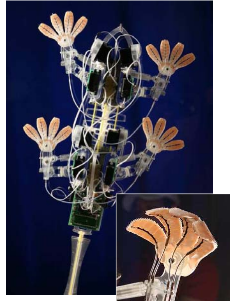
Fig. 2: Stickybot, a bio-inspired robot capable of climbing smooth surfaces. Inset: detail of toes curling to facilitate detachment
