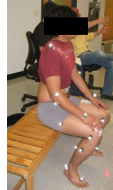
Figure 1: Marker arrangement and bench used to evaluate SitTS and StandTS
