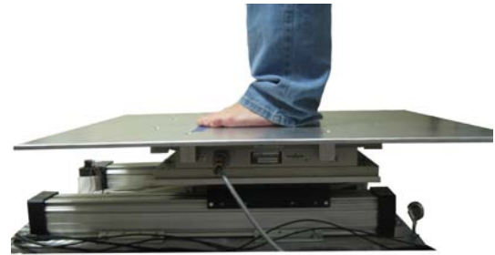
Figure 1: Experimental set-up of the pneumatic platform which translated a maximum of 0.08m forward and 0.13m backward at an average velocity of 0.25m/s. A force platform is integrated with the moving platform and used to quantify balance.
