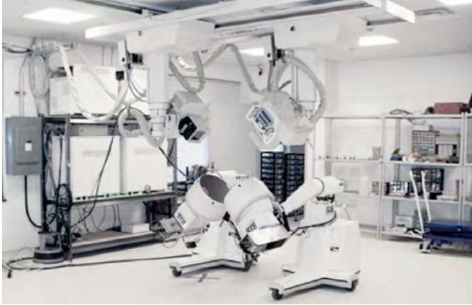
Figure 2: A large-scale biplane videoradiography system with flexible imaging configuration for animals up to the size of horses. Mobile II supports built by Radiological Imaging Services, Hamburg PA, USA ( www.risinc1.com ); X-ray system designed and integrated by Imaging Systems and Service, Painesville OH ( issi-na.com ).
