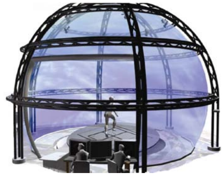
Fig. 1. The CAREN is an immersive VR system with a six degree of freedom platform with a built-in instrumented treadmill.
