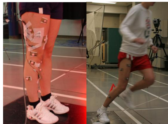
Figure 1: Experimental set up (left: placements of EMG electrodes, right: cutting on a runway).
