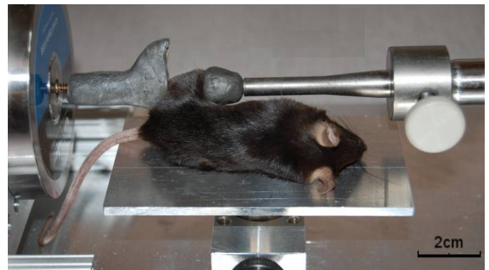
Figure 1 The loading device applies an axially-directed compressive load to the tibia of the mouse ramped load up to 15 N at 8 \mu m/s.
