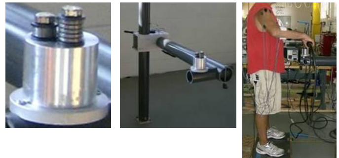
Figure 2: Joint simulator (left), configurable stand (middle) and the appearance of a male subject tested (right).
