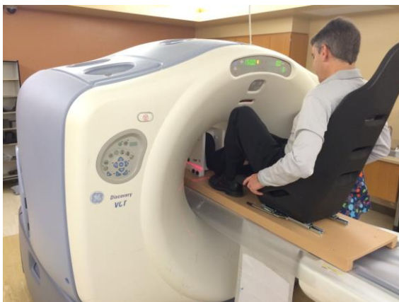
Figure 1: Device for simulated weightbearing in a CT scan. The springs (grey struts) apply a pedal load
