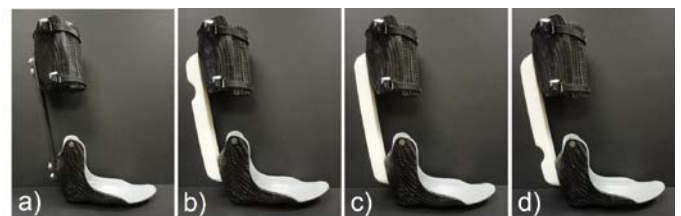
Figure 1: PD-AFO with the a) prescribed strut, b) proximal (high) bending axis, c) central (nominal) bending axis, and d) distal (low) bending axis.
