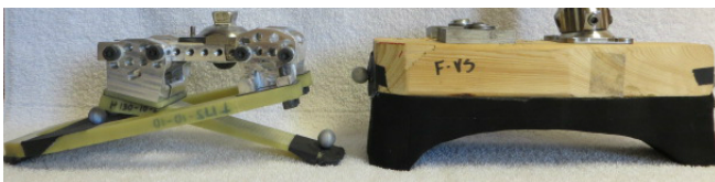
Figure 1: The energy return foot (left) and the damping foot (right).
