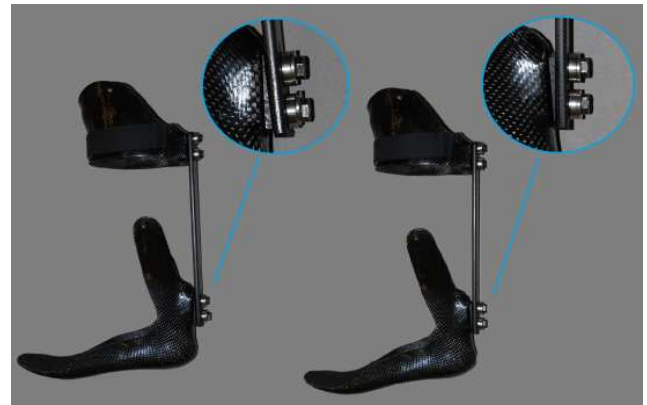
Fig. 1: IDEO in dorsiflexed condition (left) and plantarflexed condition (right). A 3° wedge between the strut and footplate changed alignment angle.
