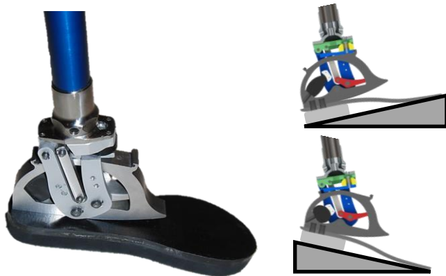
Figure 2: (Left) Photograph of the EquiFoot adaptable ankle-foot prosthesis. (Right) The EquiFoot at “foot flat” on different slopes (i.e., the time used to set the equilibrium-point of the ankle).
