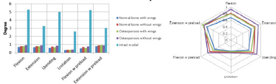
Figure 2: RoM results for L4-L5 at 10N.m for anchoring screw (with wing) and normal screw (without wing) in normal and osteoporotic bone
