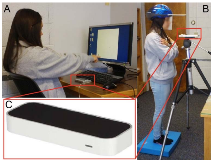
Figure 1: Test setup. For most tests (A), subjects pointed to objects on a screen while a Leap Motion sensor (C) captured their movements. In the balance test (B), subjects' head sway was extracted from the motion of dowels attached to a helmet.
