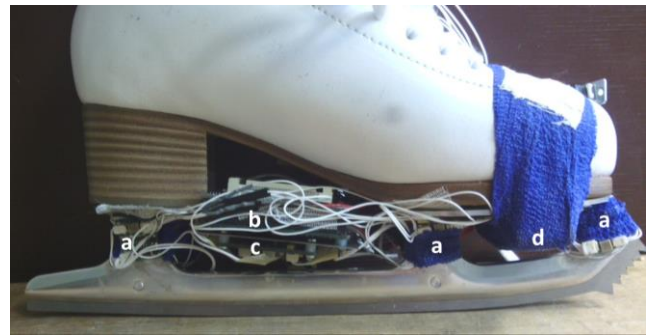
Figure 1. Instrumented blade: Wheatstone bridge boards and strain gauges (a) - front two wrapped for data collection), signal processing board (b), compact flash card slot (c), and battery (d) wrapped for data collection. Details are in [6].
