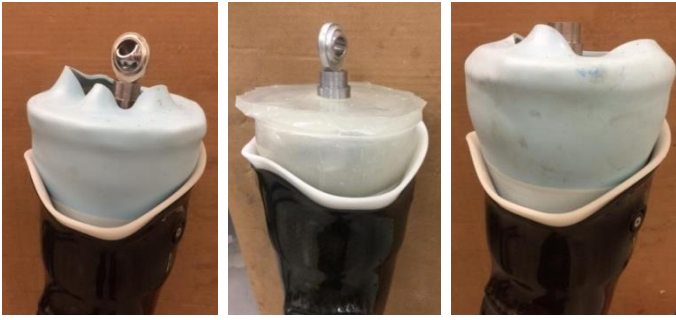
Figure 1: The three models used to simulate socket fit conditions in the benchtop testing.
