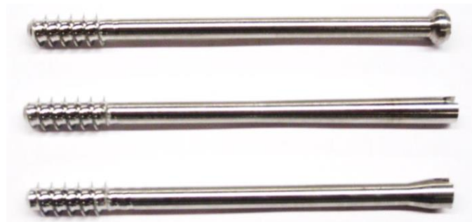
Figure 1: The three types of screws in this study are the traditional lag screw (top), long tapered screw (middle) and short tapered screw (bottom).
