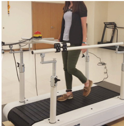
Figure 1: Subject wearing trunk sensor and ankle sensor during data collection.
