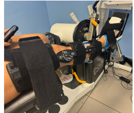
Figure 1. Experimental set-up for the measurement of barefoot passive ankle quasi-stiffness on the isokinetic dynamometer.
