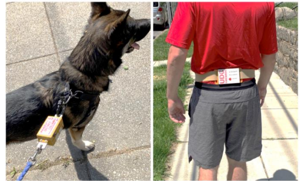
Figure 1: Leash tension (left) and gait kinematics (right) measurement systems.
