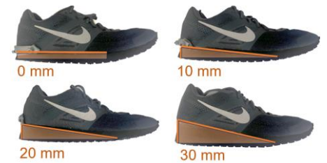
Figure 2: The running shoes we tested varied in heel-toe drop and were mass normalized with an EVA foam midsole.
