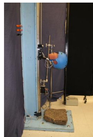
Figure 1: Skateboard helmet drop test on asphalt.
