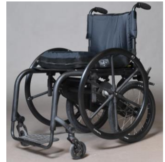
Figure 1: The experimental wheelchairs were fit with 24" Natural-Fit LT hand rims (Three Rivers Holdings LLC, Mesa, AZ).
