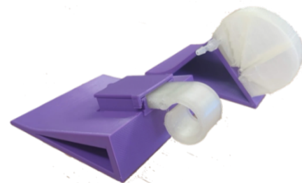
Figure 1: General design of Prototype A (left) and Prototype B (right). The prototype is positioned on the palmar side of the finger.
