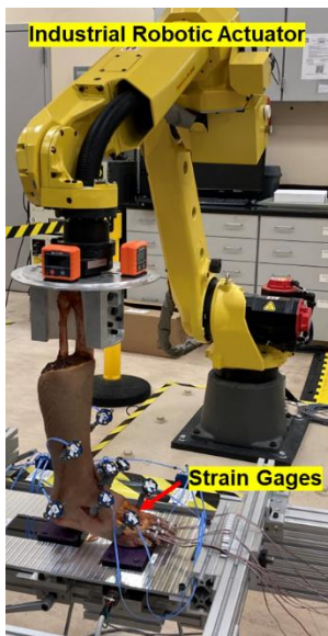
Figure 1: Experimental setup of robotic actuator and specimen.
