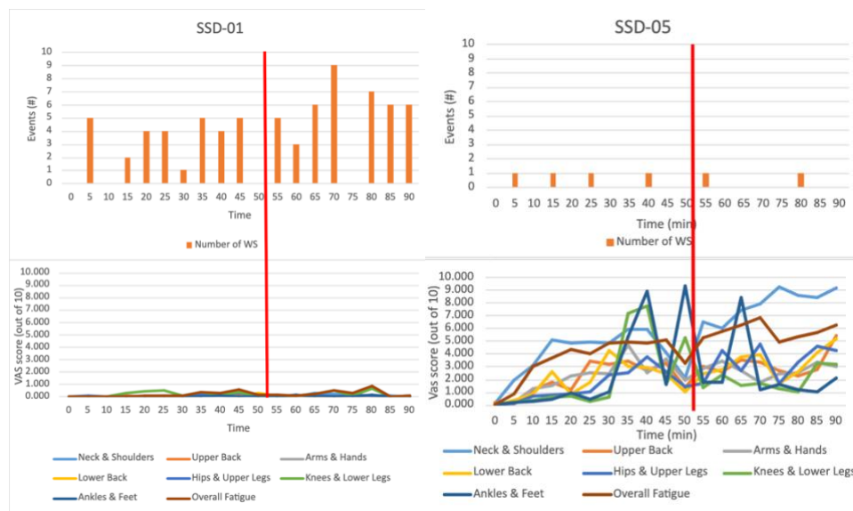
Figure 1(a and b): Subject 01 and 05 weight shifts (top) and discomfort score on the visual analogue scale (bottom) over 90 minutes. The red line indicates a break taken. Graphs in AP direction
