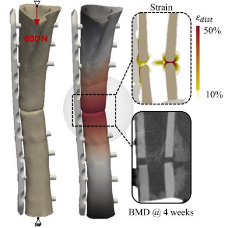
Figure 1: Interfragmentary strains were calculated in subject-specific finite element models representing each animal and mapped to downstream mineral density (BMD) in longitudinal in vivo CT scans.
