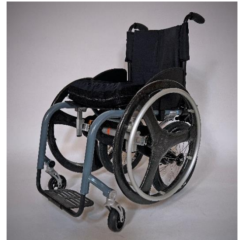
Figure 1: Chain drive experimental manual wheelchair with anterior pushrims and posterior drive wheel.
