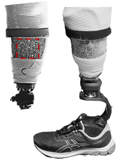
Figure 1: Anterior (left) and lateral (right) view of the residual limb donned with a speckled liner and a clear socket. The dashed red rectangle on the anterior side represents the area where DIC measured liner strains.
