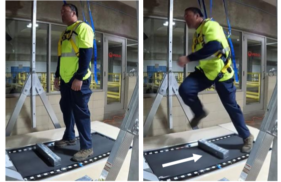
Figure 1: Reactive balance training involved using a modified treadmill to repeatedly apply trip-like perturbations. A foam block simulated a trip obstacle.
