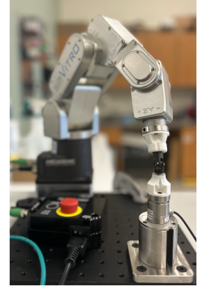
Figure 1: Robotic system for rodent joint testing.
