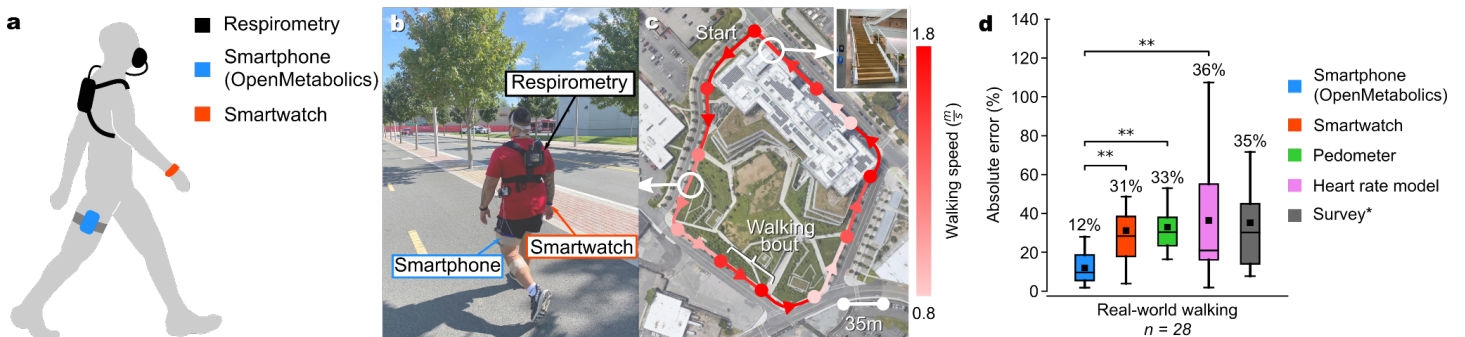
Figure 1: a , OpenMetabolics was compared with a commercial smartwatch and portable respirometry. b , Participant walking on the public sidewalk. c , Map of the 650-meter course used for real-world evaluation. Participants walked the course repeatedly, including climbing stairs each time they passed the starting point. d , OpenMetabolics significantly reduced the absolute error of the cumulative energy expenditure compared to a commercial smartwatch, pedometer, heart rate model, and self-report survey during real world walking (paired t -test, n = 28 , **P < 0.005 ).
