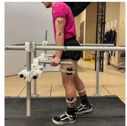
Figure 1 Instrumented subject walking with the force-sensing assistive device.
