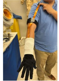
Fig. 1: Customized MoCap glove used.
