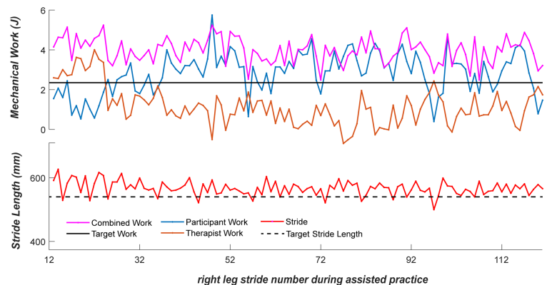
Figure 1: Exemplary data of one participant's right leg sagittal work during assisted swing for one trial (first 11 steps without DFES and assist excluded).
