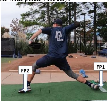
Figure 1: The instrumented pitching mound is shown with force plate 1 (FP1) under the drive leg and force plate 2 (FP2) under the stride leg.
