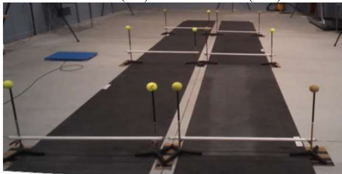
Figure 1: View from the start of the obstacle course. Six obstacles spaced 3 m apart. Participants walk the right side (12 m) to the end of the walkway, come back on the left side, and repeat. During OP, participants stand 0.3 m past the first obstacle and match their foot to the height of the second obstacle 2.7 m away.
