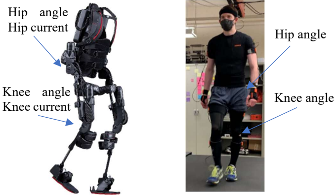
Figure 1: (Left) The EksoGT and its associated onboard signals. (Right) The XSens inertial motion capture suit and its associated signals.
