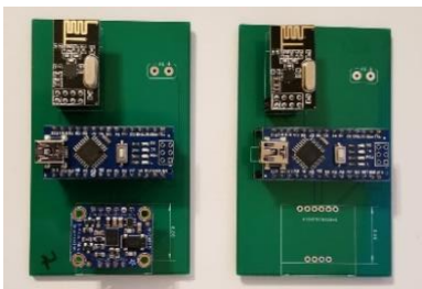
Figure 1: IMU device (Left) that transmits the orientation data back to the receiver/hub (right) for processing data in python.
